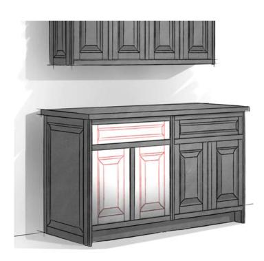
INSET Door/Drawer panels are installed within the faceframe.
